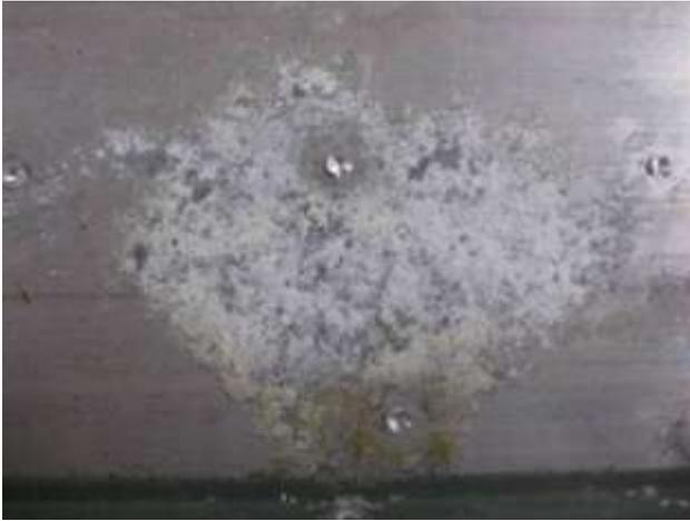
The two doublers. The aft side had more corrosion than the forward side.
